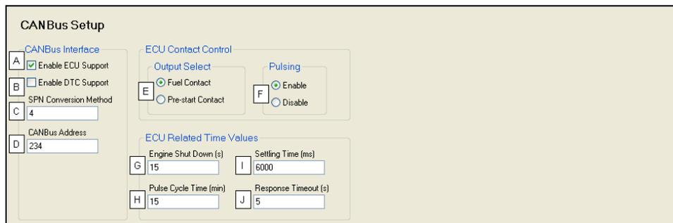
Figure 4-21. CANbus Setup
