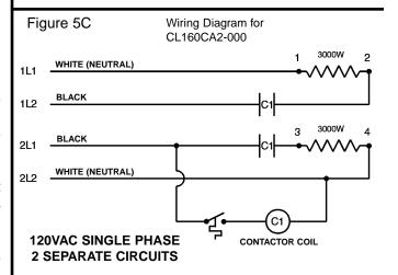
CONTACTOR MUST BE USED DUE TO HIGH AMPERAGE (TYPICAL WIRING DIAGRAM SHOWN)
