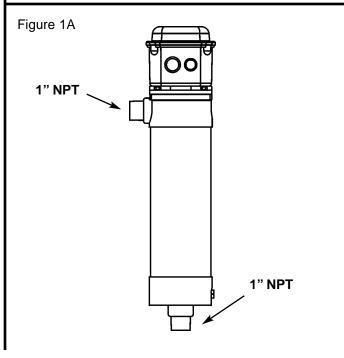
After mounting, plumbing, and wiring the heater, refill the engine with coolant (energizing the heater without coolant may cause element failure). It is recommended that the engine be operated after plumbing the heater to eliminate possible air pockets in the water jacket. Prior to energizing the heater, the thermostat setting can be adjusted by removing the electrical enclosure cover and rotating the knob to the desired setting (see Figure 6).
