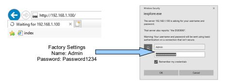
4. It is now possible to view and configure the DSEGateway<sup>®</sup>. Make a note of the DSEGateway<sup>®</sup> ID number. This is required when adding the DSEGateway<sup>®</sup> to DSEWebNet<sup>®</sup>.
