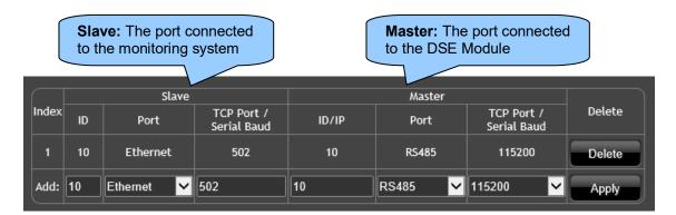
Index 1 is receiving MODBUS requests from the external monitoring system on **Ethernet, TCP Port** 502
