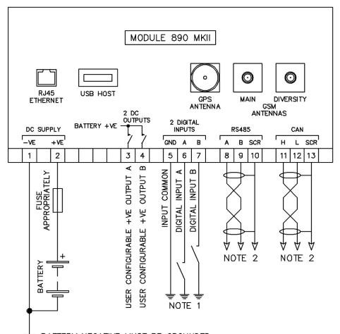
NOTE 2. IF THE MODULE IS FIRST OR LAST UNIT ON THE LINK, IT MUST BE FITTED WITH A 120 OHM TERMINATION RESISTOR ACROSS THE A AND B OR H AND L TERMINALS.
